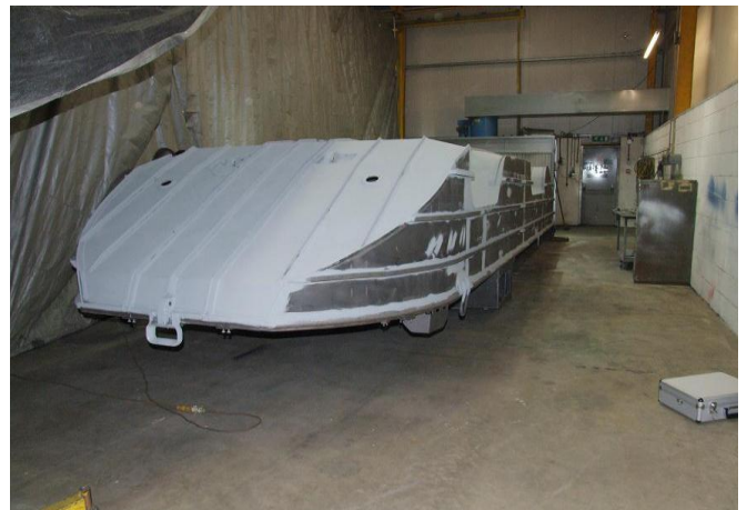
Bodywork blast-cleaned and Zinga applied to underside
