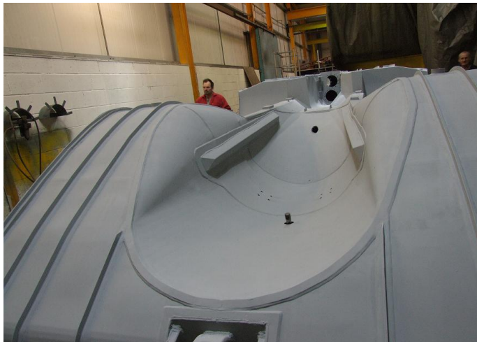
A view of the prop-shaft tunnel where the back axle is seated
