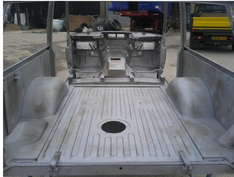
Body-shell is blast-cleaned
